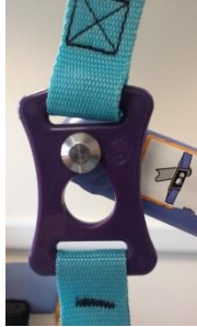
Sling fixing clip attached to hoist spreader bar lug (stud) in the correct position
