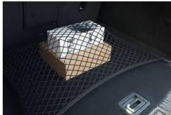
Examples above of vehicle netting which can secure equipment and also provide protection to the front of the vehicle if a boot shelf cannot be used .
