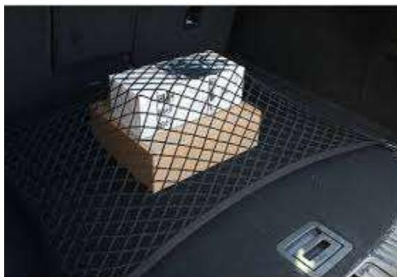
Examples above of vehicle netting which can secure equipment and also provide protection to the front of the vehicle if a boot shelf cannot be used .
